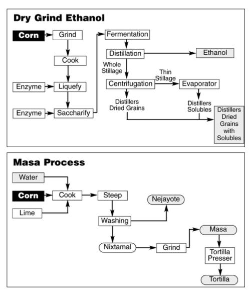
Figure 2: The main corn refining processes and products (Iowacorn<sup>4</sup>)
